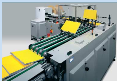
Alternate (head to foot) delivery and shingled exit onto an exit belt for easy take off the bound products.
