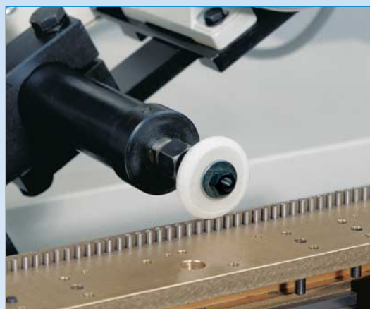
Pin grinding in one working operation
