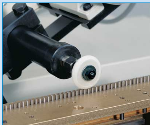
Pin grinding in one working operation
